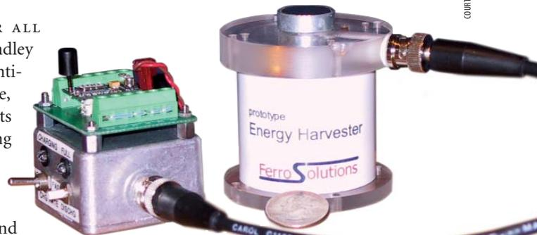
A new device uses vibrations to power a sensor.
